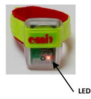
It is the competitor's responsibility to ensure that their emiTag has been correctly activated at the Start and that a correct 'punch' has been recorded at each control, by checking that the emiTag LED flashes.
