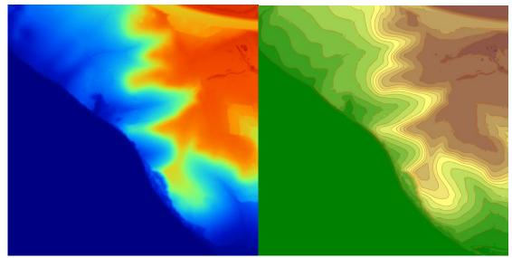
The left slide shows a basic altitude heatmap -1 million readings at  $1m^2$  spacing – blue low, red high. The right slide shows more familiar colours, grouped in 2.5m altitude ranges with smoothed contours overlaid.
