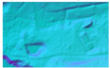
Adding "micro contours" at eg 10cm intervals can highlight knolls etc, but don't over-detail the final map!!
