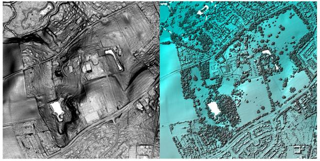
These last two are a "slope gradient" template where steeper ground is shown in darker colours, and a hillshade template obtained from a DSM dataset. This picks out hedges and walls well. I haven't used these, but other mappers have found them useful.
