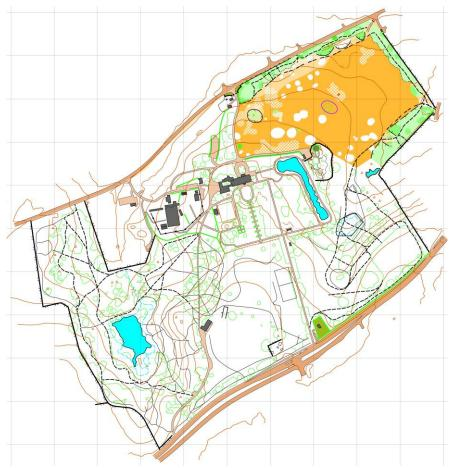
This shows an example of the base map I take out into the field. A small section is already completed. I've drawn with "proper" symbols all the features I'm pretty confident are correct – eg because they are confirmed on at least two templates. I've used "drafting" symbols – eg thin lines of different colours – for features that I'm not confident in – for example because they are suggested by only one template.
