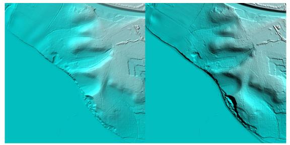
The left hand template is created with the "virtual sun" in the NW, and the right hand with the "virtual sun" in the NE. Composite images are also possible.
