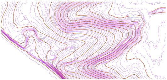
The smoothed 2.5m contours are generated in vector format. Here, I've imported these and opened 0.5m interval contours as a template beneath. Some mappers always trace the contours over a template, but I find importing and adjusting pre-smoothed contours is normally quicker. An obvious area for adjustment is the pronounced gully at the head of the valley.
